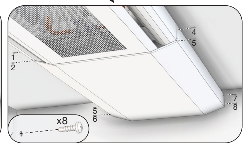
CW cover installation, inserting screws. Screws (x8) included.
