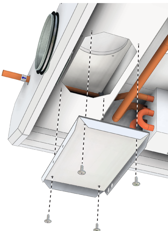
Picture 20. Opening inspection hatch.
