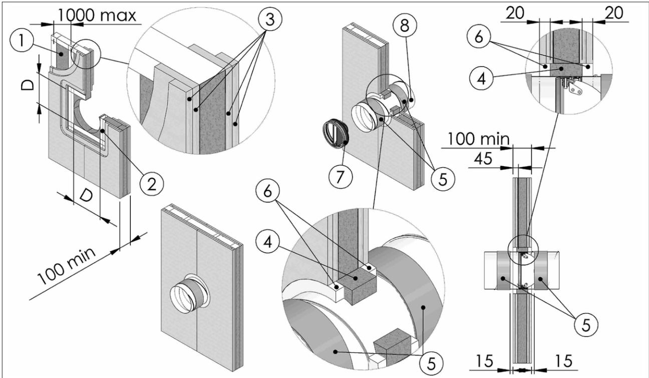
**Model FBC4 - FBC7: circular hole, plasterboard and rock wool sealing**
