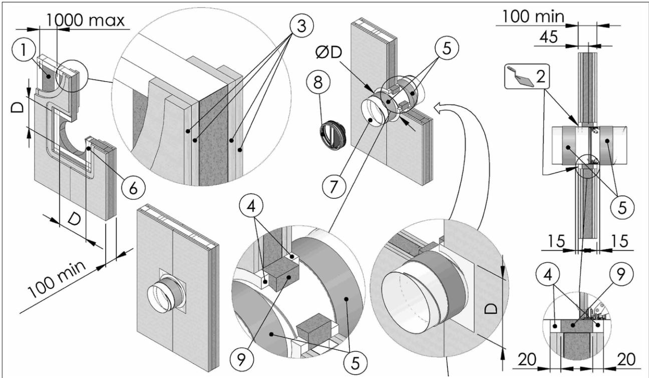
**Model FBC4 - FBC7: square hole, mortar or plaster putty sealing**
