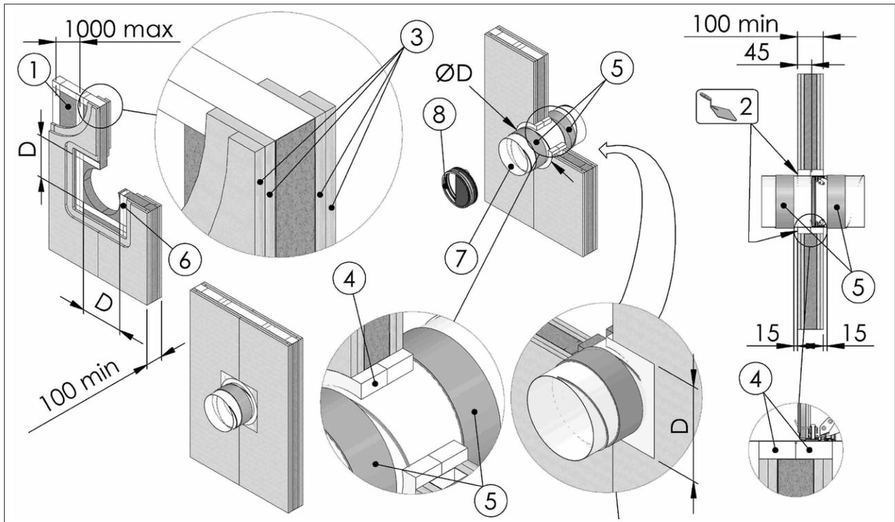
**Model FBC4: circular and square hole, mortar or plaster putty covered rock wool sealing**
