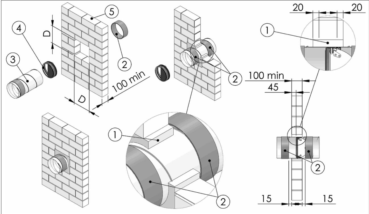
**Model FBC1: square hole, mortar or plaster putty covered rock wool sealing**
