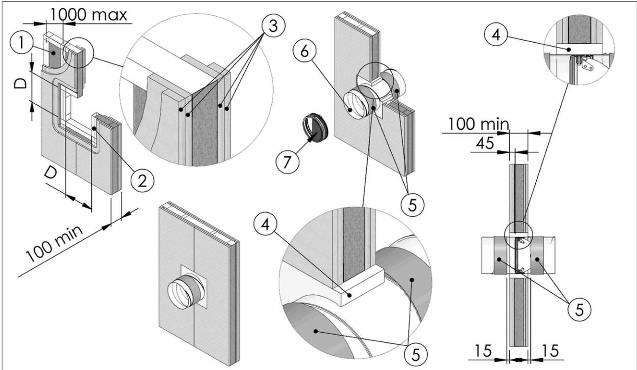
**Model FBC4 - FBC7: square hole, mortar or plaster putty covered rock wool sealing**
