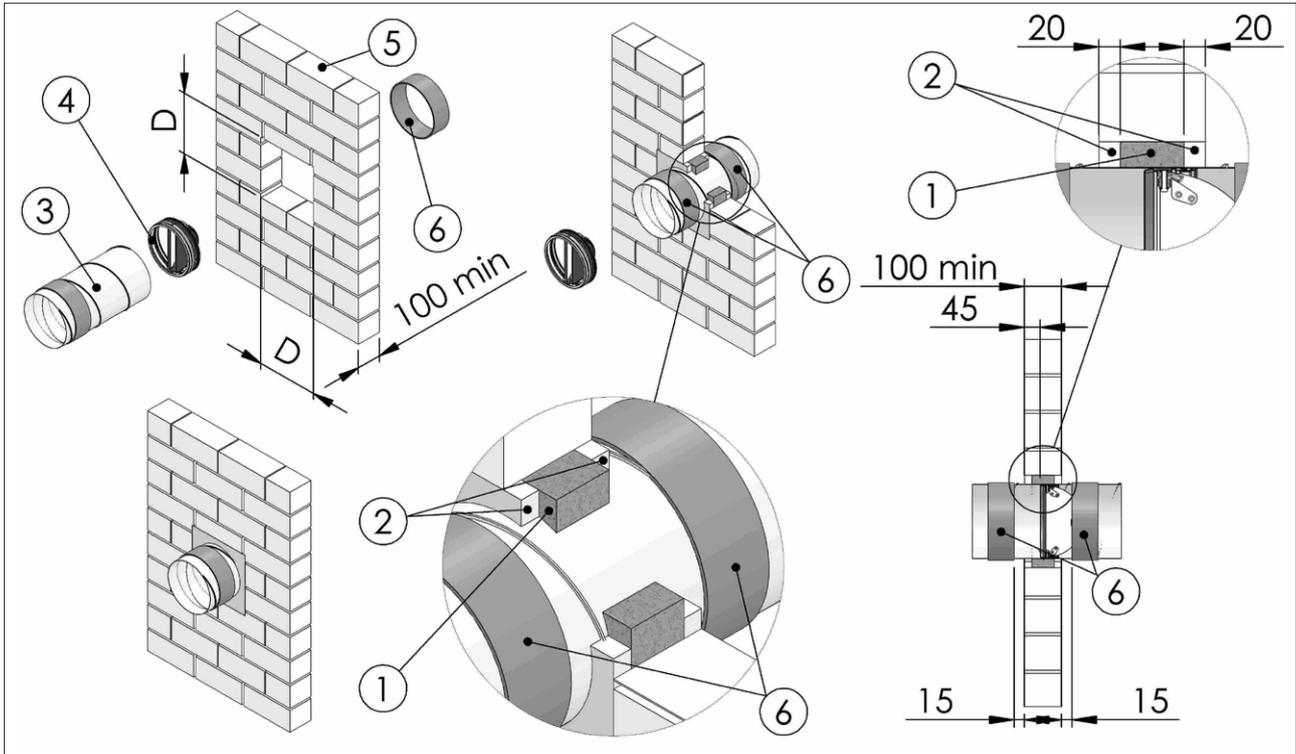
**Model FBC4 - FBC7: square hole, plasterboard and rock wool sealing**
