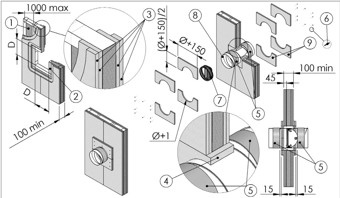
**Model FBC4 - FBC7: circular hole, mortar or plaster putty sealing**
