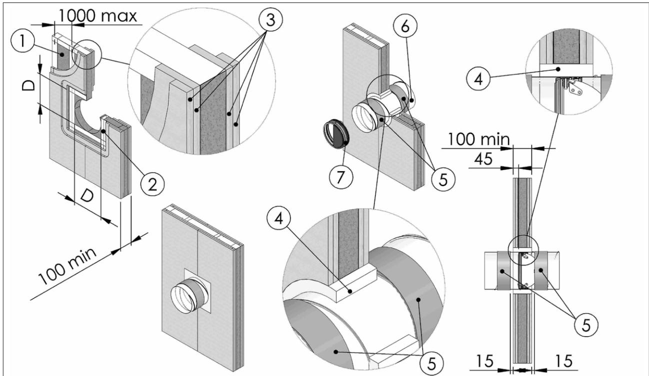
**Model FBC4 - FBC7: circular hole, mortar or plaster putty covered rock wool sealing**
