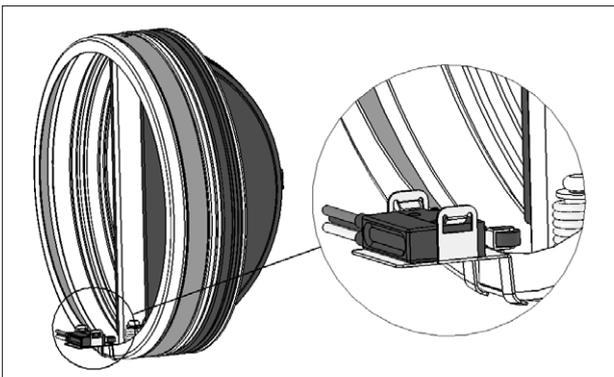
**Temperature calibration of thermosensitive element for automatic damper closing**
