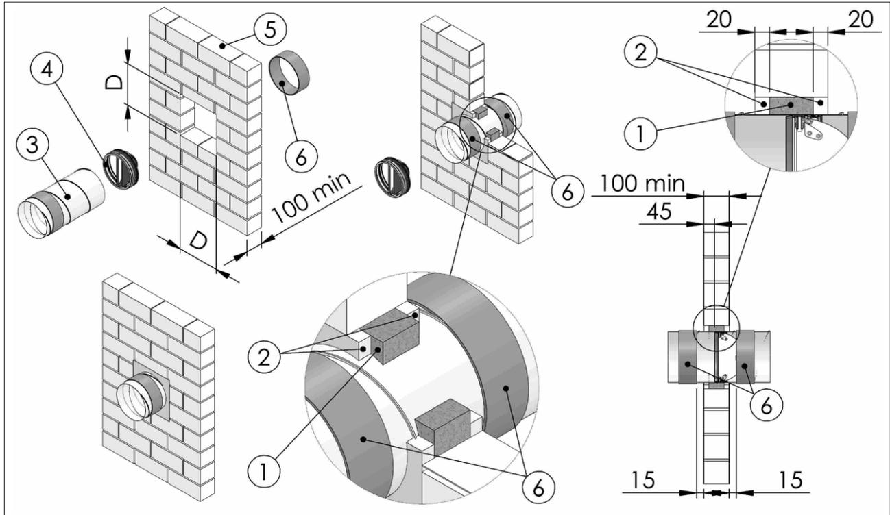
**Model FBC1: square hole, plasterboard and rock wool sealing**
