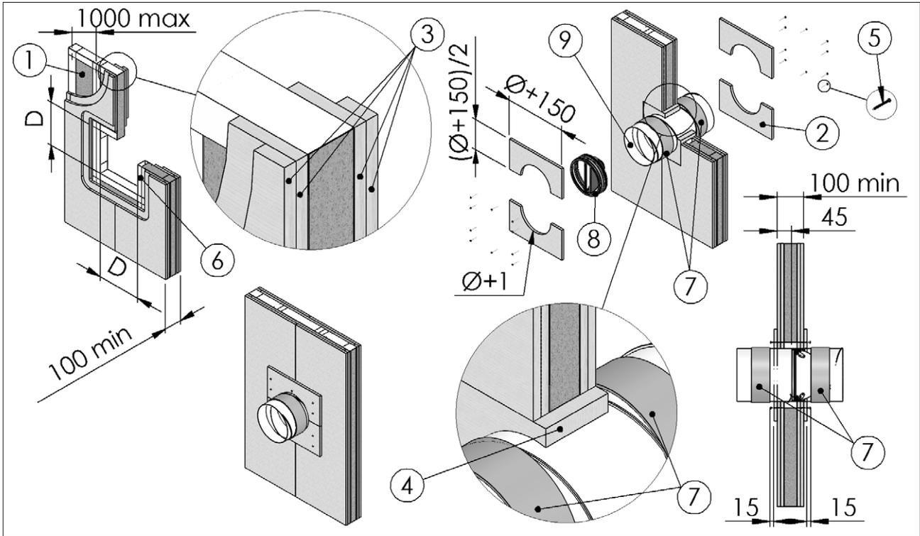
**Model FBC1: circular hole, mortar or plaster putty sealing**
