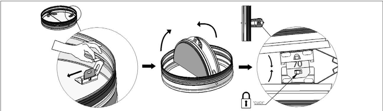
The fire damper is equipped with a spring for closing the blade: pay attention to the hands.
