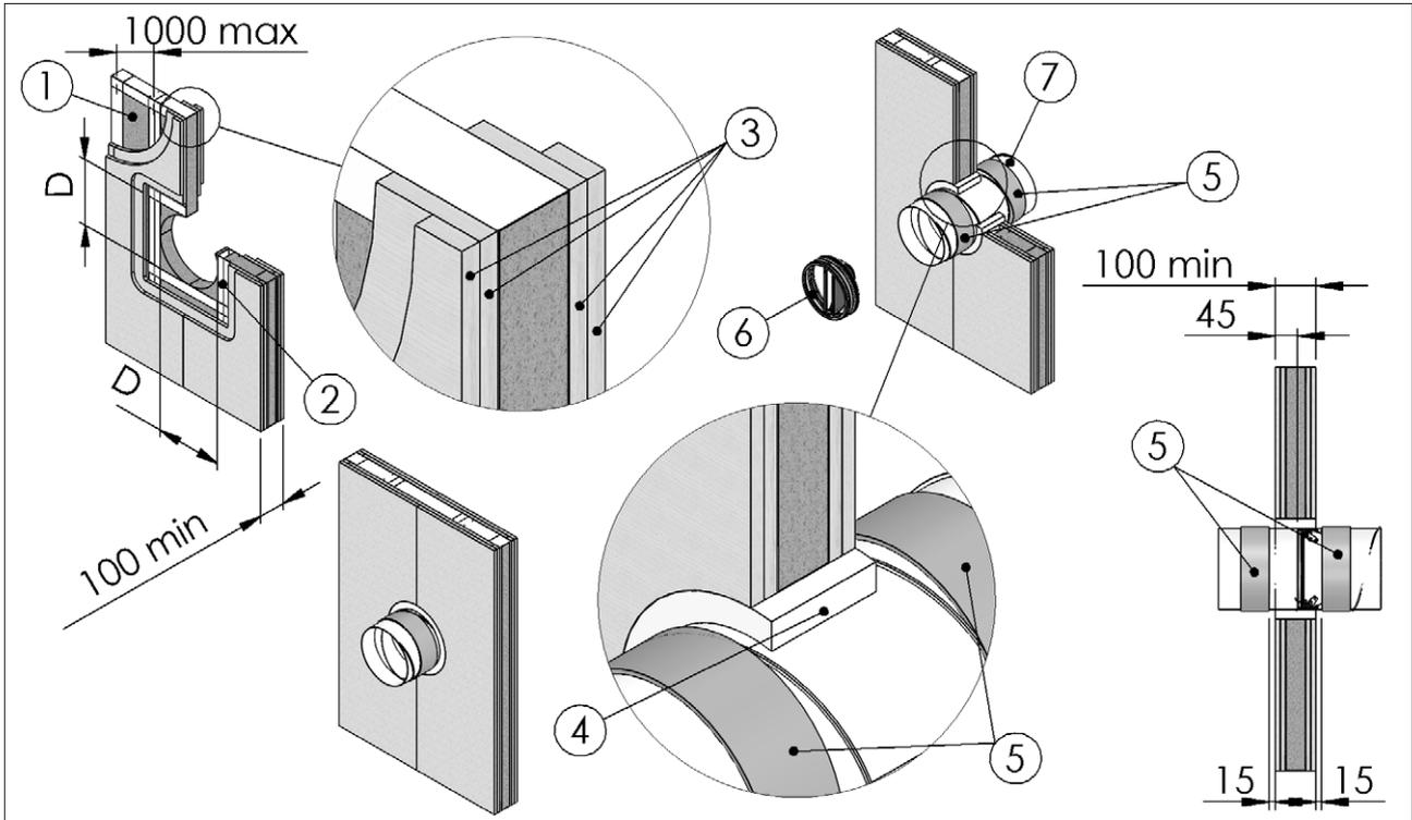
**Model FBC4: circular and square hole, mortar or plaster putty sealing**
