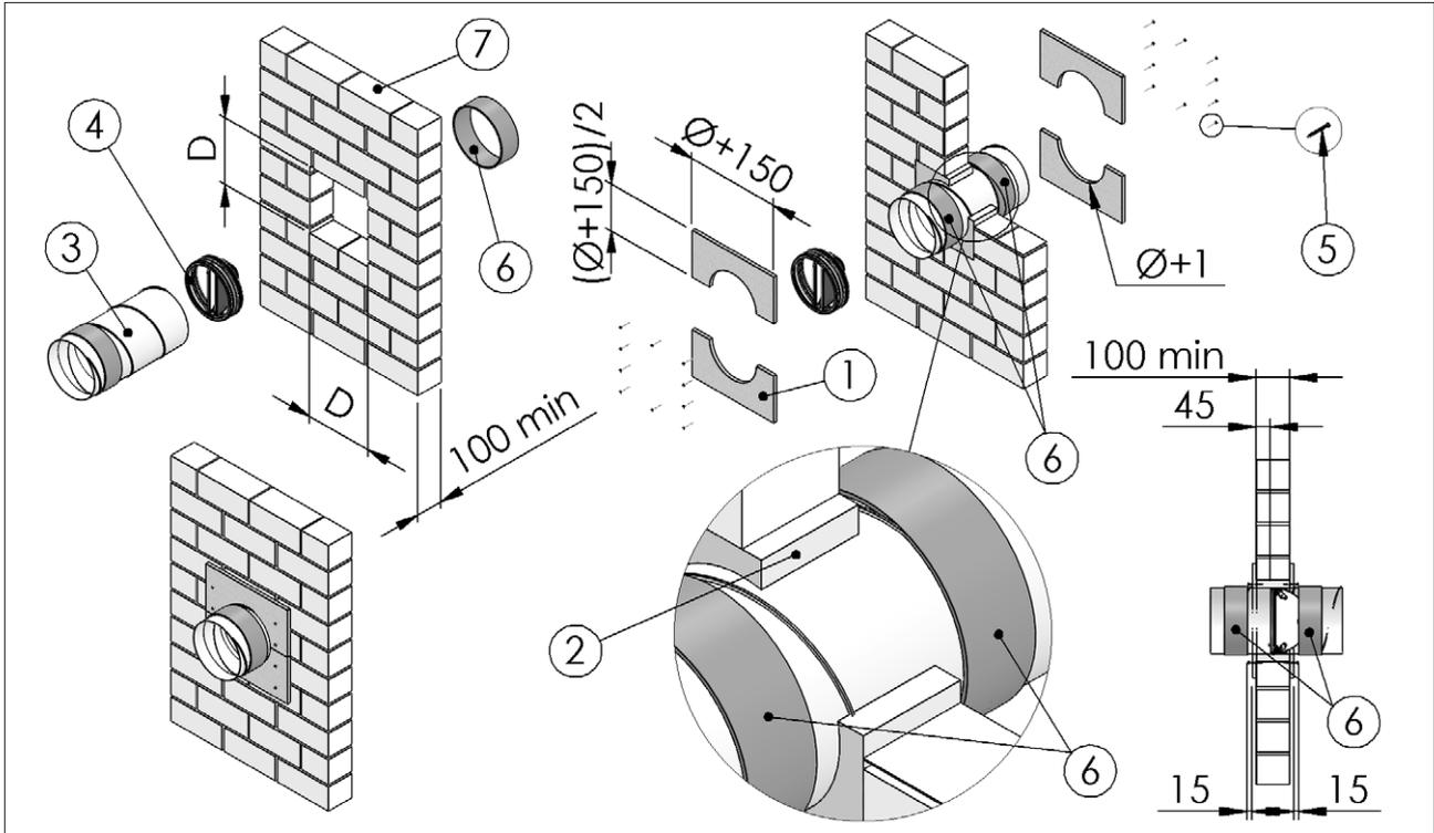
**Model FBC1 - FBC4 - FBC7: circular hole, mortar or plaster putty sealing**
