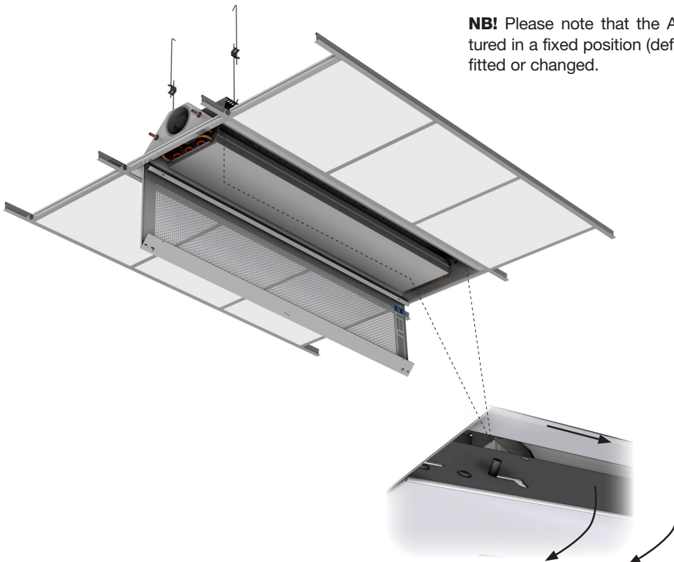
Picture 3. When the faceplate is lowered or removed, the battery is accessible from below.
