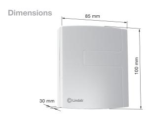
The sensor is mounted in the cover-part of the casing. The cover is easy to detach from the back by means of snap-in grips and detachable terminals. This makes mounting easier. Furthermore, no cables have to be disconnected, which simplifies service and replacement.
