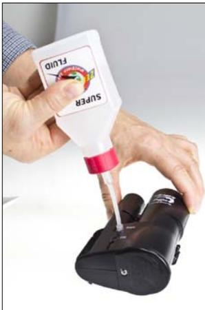
Fig. 16: Suction of the excess fluid
