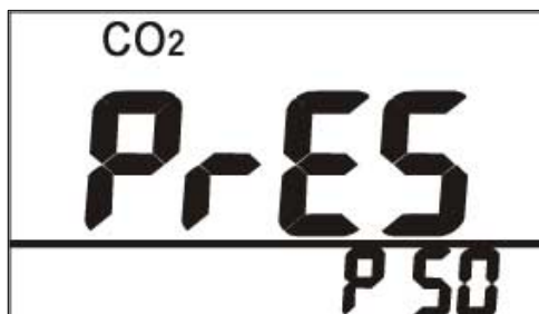
Fig. 23: Setup - air pressure, Display 1
