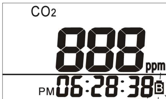
Fig. 3: Display with low battery indicator
