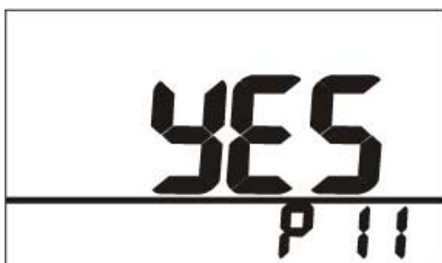
Fig. 18: Setup - Delete all records, Display 2
