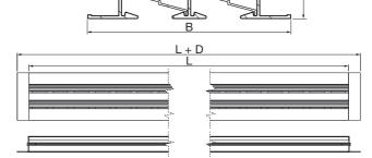
Both ends are equipped with flanges.
