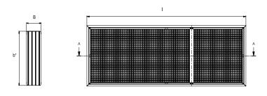
$b^* = Manufactured$  height of splitter is b-5 mm, to fit into duct.
