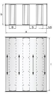
Length of splitter should be 50 mm shorter than length of duct.
