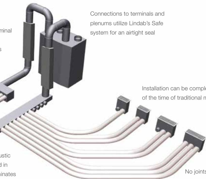
Connections to terminals and plenums utilize Lindab's Safe system for an airtight seal
