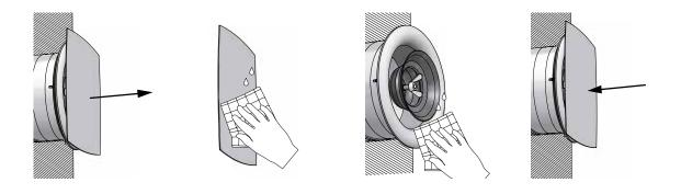
To clean the valve remove the front plate and clean it with a mild detergent or a wet cloth.
