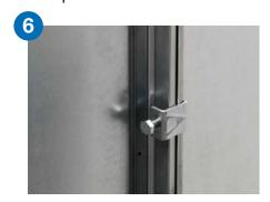
Assemble the Rectangular Joint Bolt Clamp RJBC over the flanges. To reach air tightness class B it is enough to have a distance of 700mm between the clamps. To reach air tightness class C a maximum distance of 400 mm is allowed.
