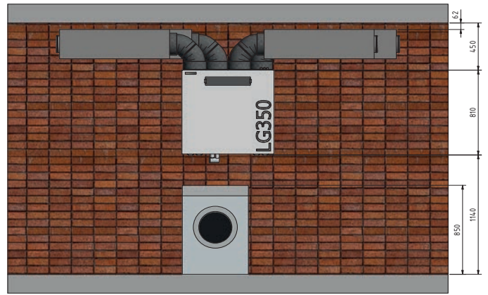
Wall-mounted installation with air exchange silencers
